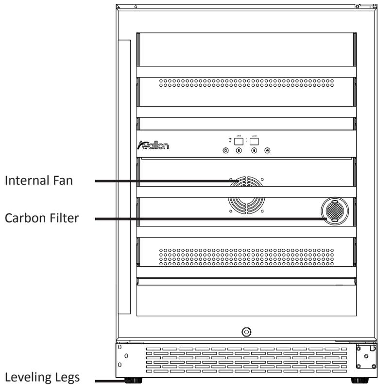
Note: The carbon filter should be replaced every 3-6 months depending on the unit's exposure level to odor. If the unit is placed in kitchen regular replacement every 3 months is ideal.
