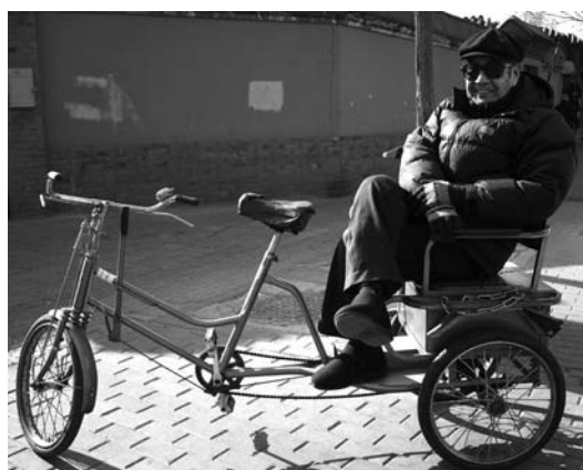
Figure 6: Street view of intergenerational transport in Beijing. This image shows an adapted bicycle functioning as wheelchair attached to a bicycle which also can be un-clipped from the bicycle. Photo: STC/Shannon Bufton
