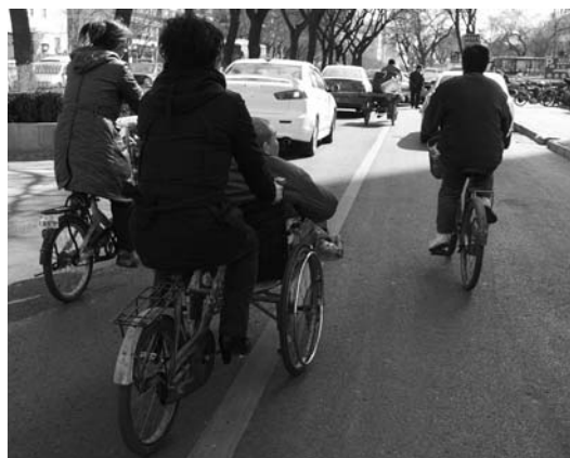
Figure 5: Mobility for the elderly with the tricycle in Beijing. The bicycles used are highly adapted to service the transport of elderly people. The vehicle is equipped with a comfortable backseat and a lockable container. Photo: STC/Shannon Bufton
