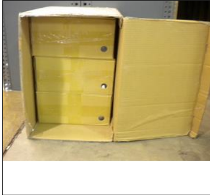
Example of taping a 2 piece shoe box using 2 inch tape around both length and width of shoe box.
