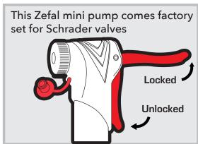
First identify what style valve stem the bicycle has. Then set the internals of the pump head to match the bicycle's valve. Unthread the metal cap on the pump head opening and remove the internal parts.
