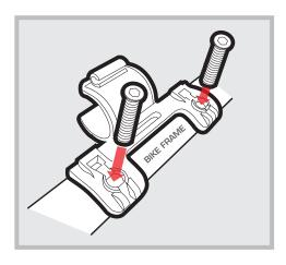
Use included screws to mount to frame using existing water bottle location on non-drive / left side of bicycle. For use with water bottle cages.
