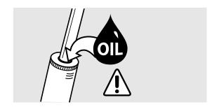
Periodically lubricate the pump barrel with a couple of drops of oil.
