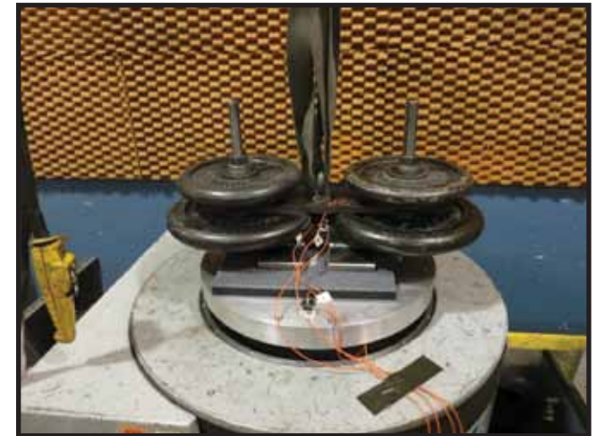
Shock transmissibility test setup under 220 pounds.
