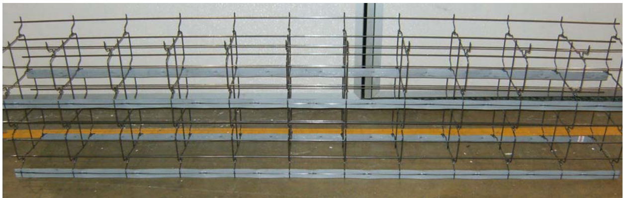
Photograph No. 2: Showing a linked wire mesh web of an insulated concrete form sample.
