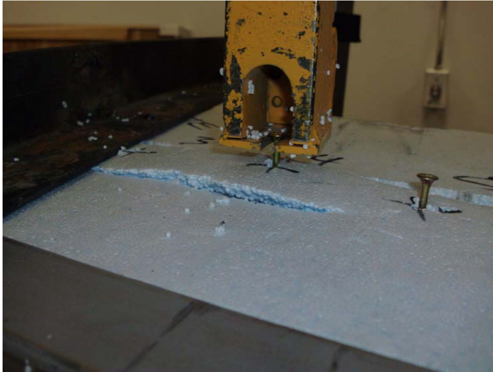
Photograph No. 3: Showing test set-up for screw and nail withdrawal test using Satec Unidrive Testing Machine.
