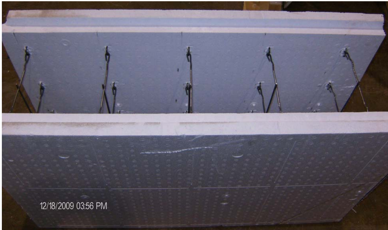
Photograph No. 1: Showing a typical insulated concrete form sample.
