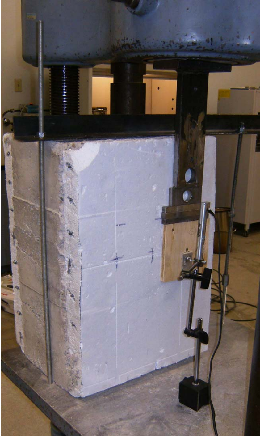
Photograph No. 4: Showing set-up for lateral fastener resistance tests.
