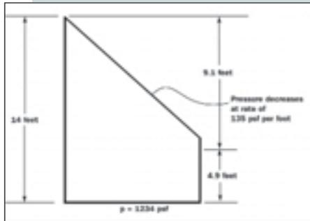
admixture. From Table 3, the base pressure value is 1060 psf. From Table 1, the weight coefficient is 0.5 ( $1 + w/145$ ), or 0.5 ( $1 + 135/145$ ) = 0.97. The chemistry coefficient  $C_c$  is 1.2 for Type I cement used with a retarder. The maximum pressure, therefore, is  $1060 \times 0.97 \times 1.2 = 1234$  psf.
