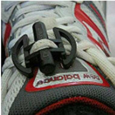
Figure 2: Passive RFID Tag – marathon race chip. Source: Yoppy used under CC BY
