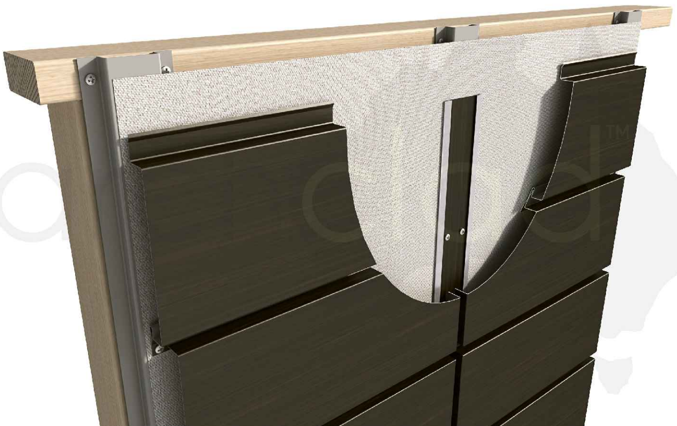
DETAIL - W4 (HORIZONTAL WALL PANEL VERTICAL JOINT FLASHING - PLAN)
