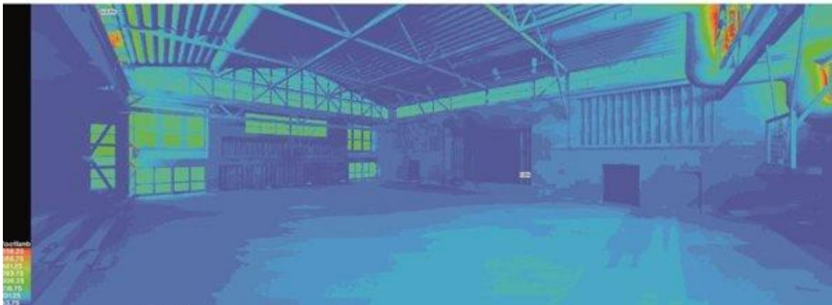
*A clear indication of how specifying the right glass product can negate heat and glare gain. Product: Okalux Kapilux – Capillary Daylighting*
