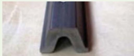
Extruded shapes allow a continuous length to be produced and docked to length. Intricate profiles can be made, including hollow sections. However the shape must conform to a predominately two dimensional form unless machined after processing.
