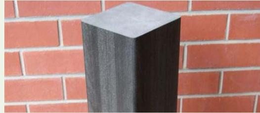
Fine ground wood flour is added to the recycled content mix during processing at the rate of up to 50%. It adds stiffness (increases the modulus of elasticity). This material is also called wood plastic composite.
