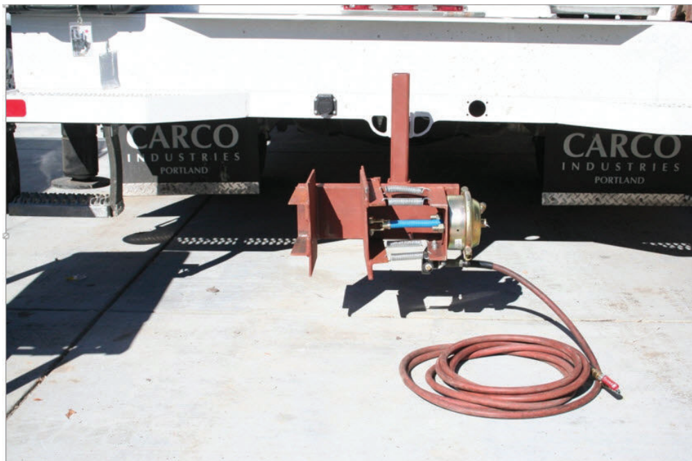
Figure 4. Pneumatic vise designed to capture the front tire of the test motorcycle.
