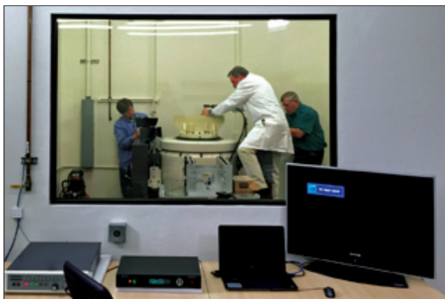
Figure 7. Control room with view of shaker room; note remote SCU, controller, PC and large monitor on desk.
