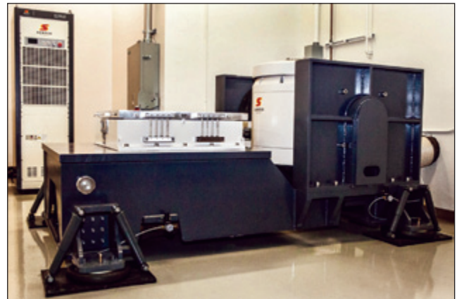
Figure 2. Advanced vibration testing system including horizontal slip table and large vertical/horizontal tip-over shaker sharing foot-isolated mono-base.
