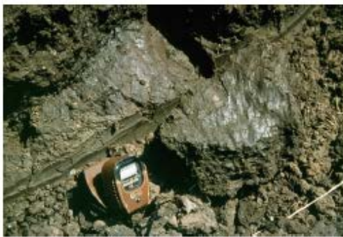
Fig. 4 Slickensides are polished, grooved surfaces caused by the surfaces sliding against each other during shrinking and swelling of the soil. Credit: Soil Science Society of America
