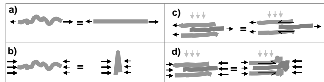
Fig. 3. Schematics - Individual and interacting peat particles under tensile and compressive stresses.
