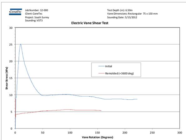
Figure 6. Electric VST from 6.5 m depth.
