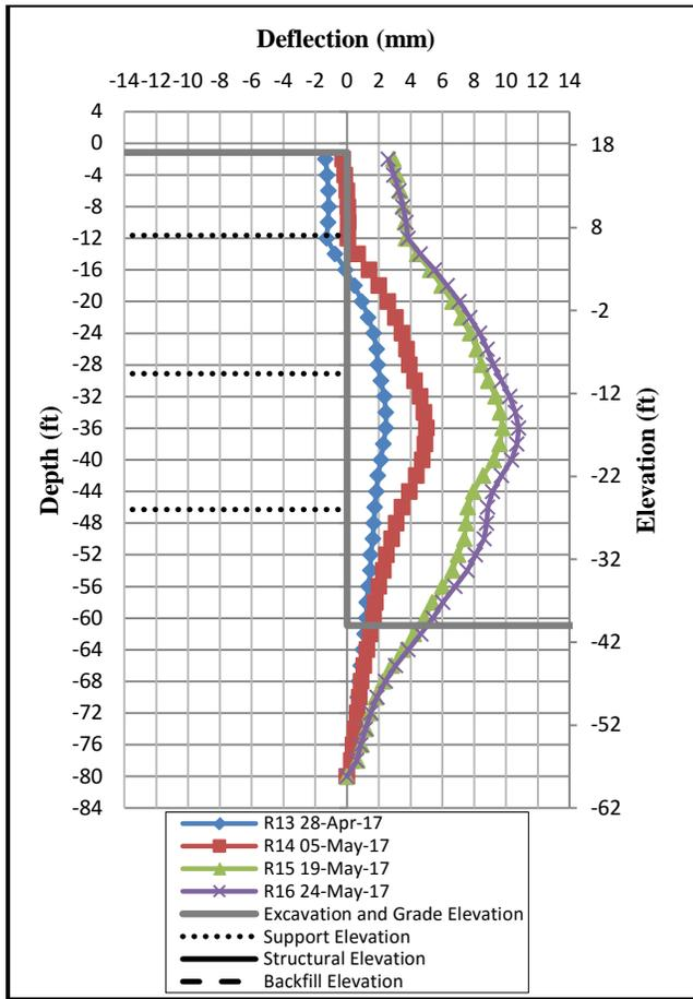
**Fig. 11.** Inclinerometer Readings for Hybrid Shoring Wall 1 – CSM Panel
