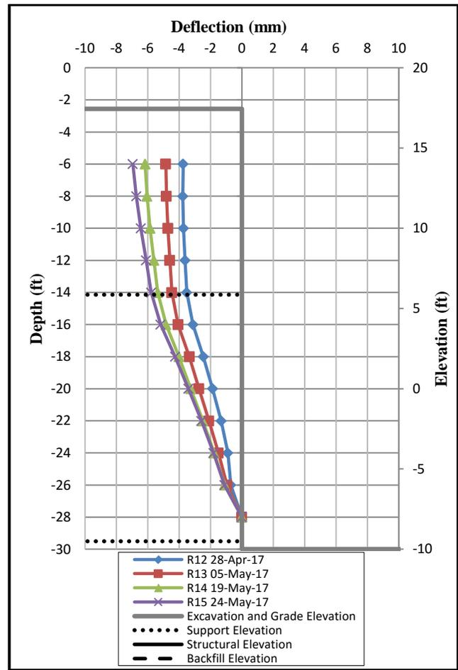
**Table 2.** Comparison of Inclinerometer Monitoring Data with Pile Target Survey Data for Hybrid Shoring Wall 1
