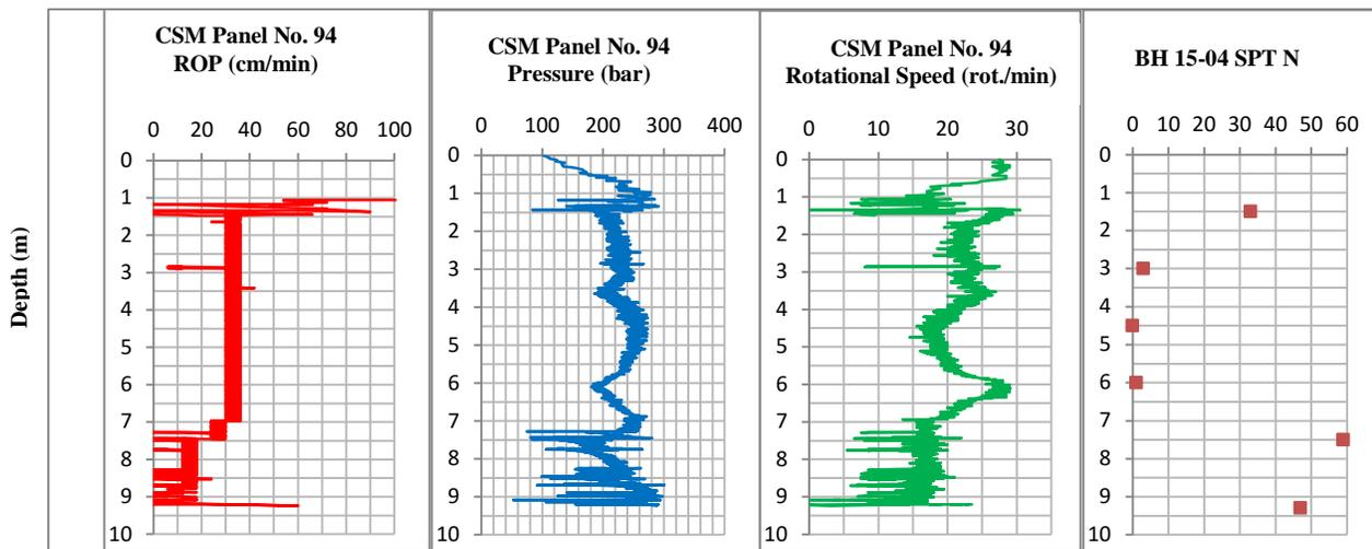
Fig. 7. Hybrid Shoring Wall 2 typical CSM output parameters compared with SPT N values
