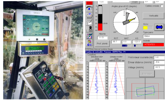
Fig. 15. Verticality controls available to the grab operator.
