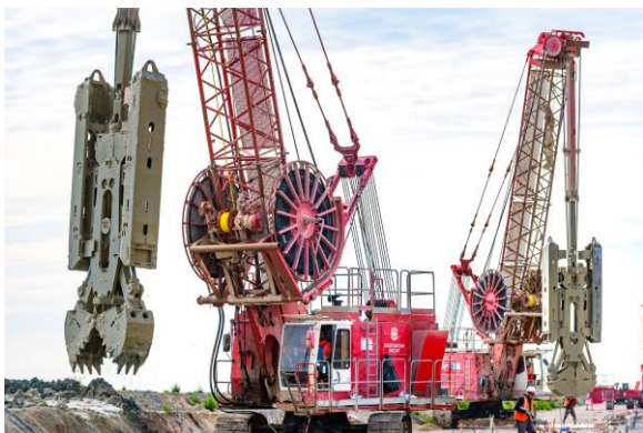
Fig. 14. Hydraulic grab for diaphragm wall excavation.
