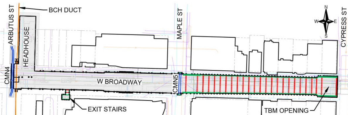
Fig. 2. Arbutus Station and Double Crossover Plan.
