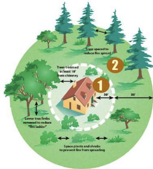
Figure 9. Defensible space zones around structures. 28
