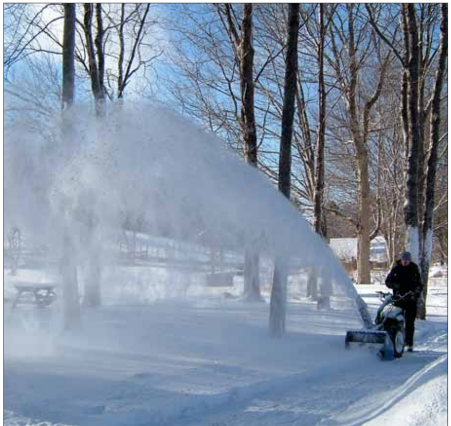
A snowblower attachment makes the BCS tractor useful year-round. Maintaining one machine instead of several is a distinct advantage.
