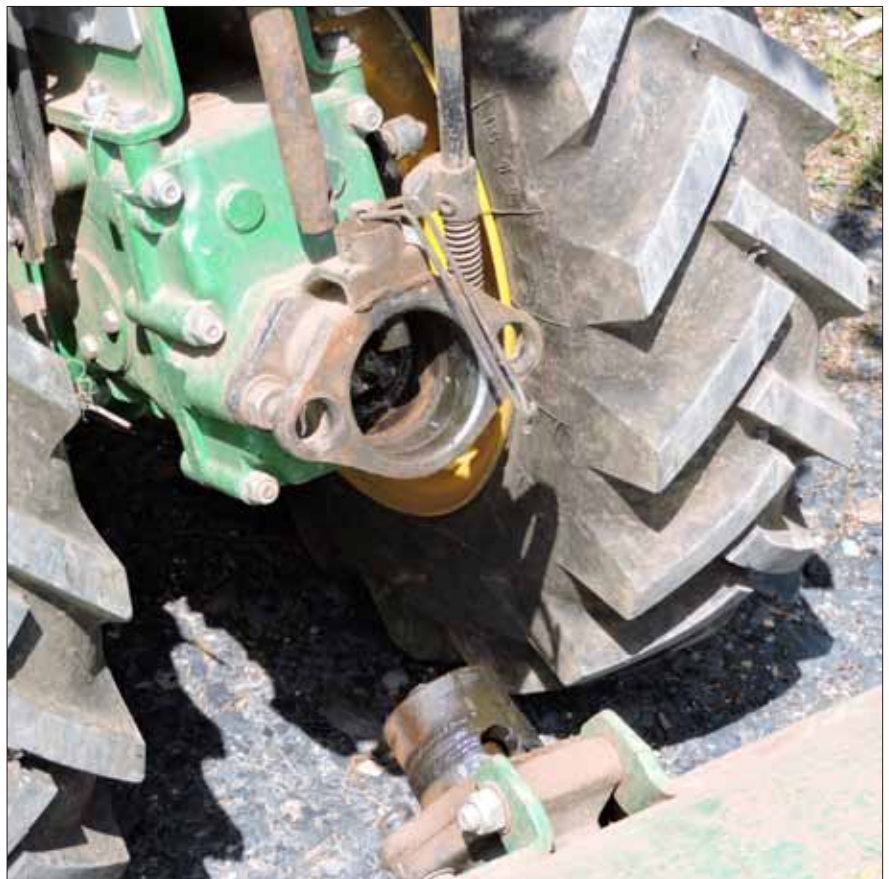
There's just one PTO (power take-off) coupling on the machine, but reversible handle-bars allow for the operation of front or rear implements.
