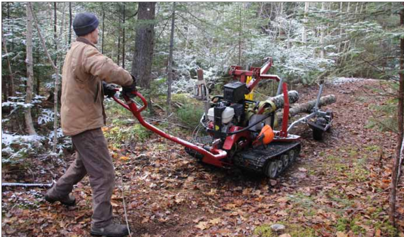
The IronHorse, a nine-horsepower tracked machine, serves well for extracting wood, and causes very little ground disturbance.
