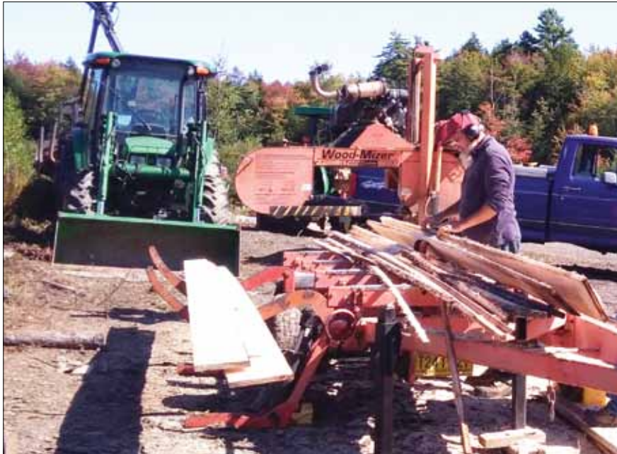
Roger Zinck was on hand generating some lumber with his Wood-Mizer LT40 portable bandsaw mill.
