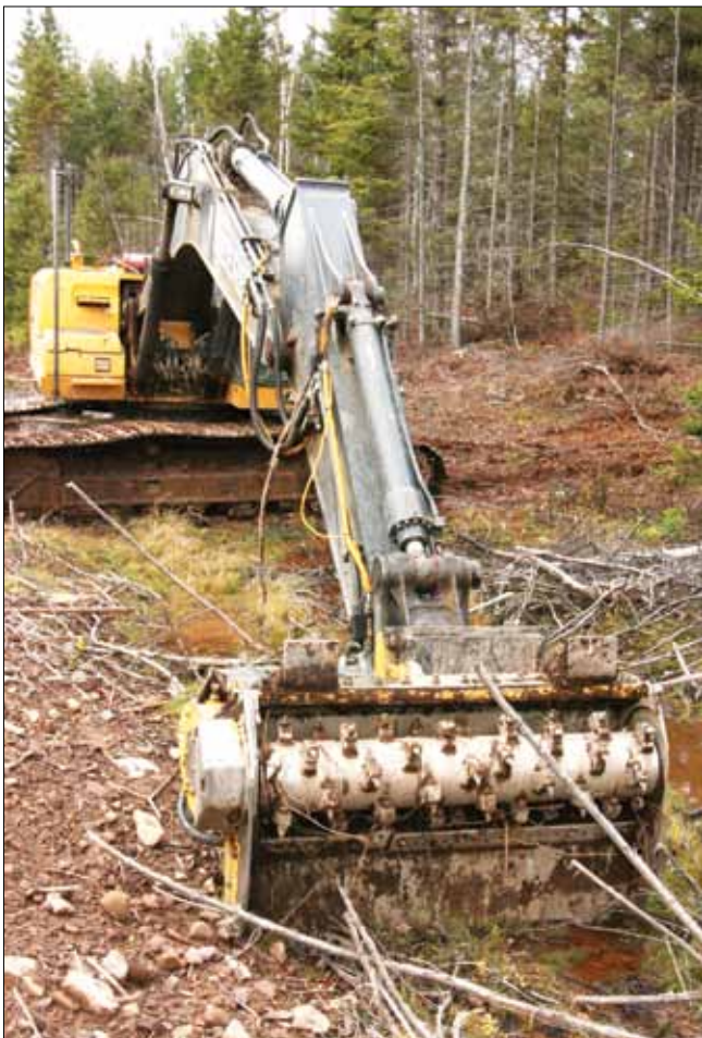
One of the machine demos featured a mulching head used to scarify partial-cut sites in preparation for underplanting.
