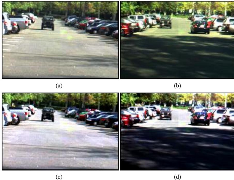
Fig. 3. Example RGB images of vehicle driving towards camera in the morning (a) and afternoon (b) along with the corresponding images after pre-processing with IAR (c), (d).
