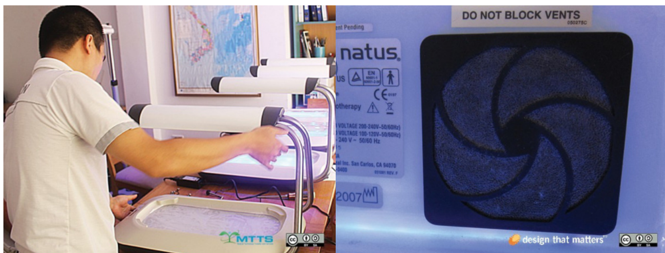
Left: Firefly manufacturer MTTs submits a series of new Firefly devices to the “burn-in test” at their offices in Vietnam. Photo courtesy Michael O'Brien of MTTs. Right: The vent for the Natus NeoBlue LED Overhead Phototherapy, one of the most popular phototherapy devices used in the United States. An internal fan helps move air through this vent to cool the electronics.
