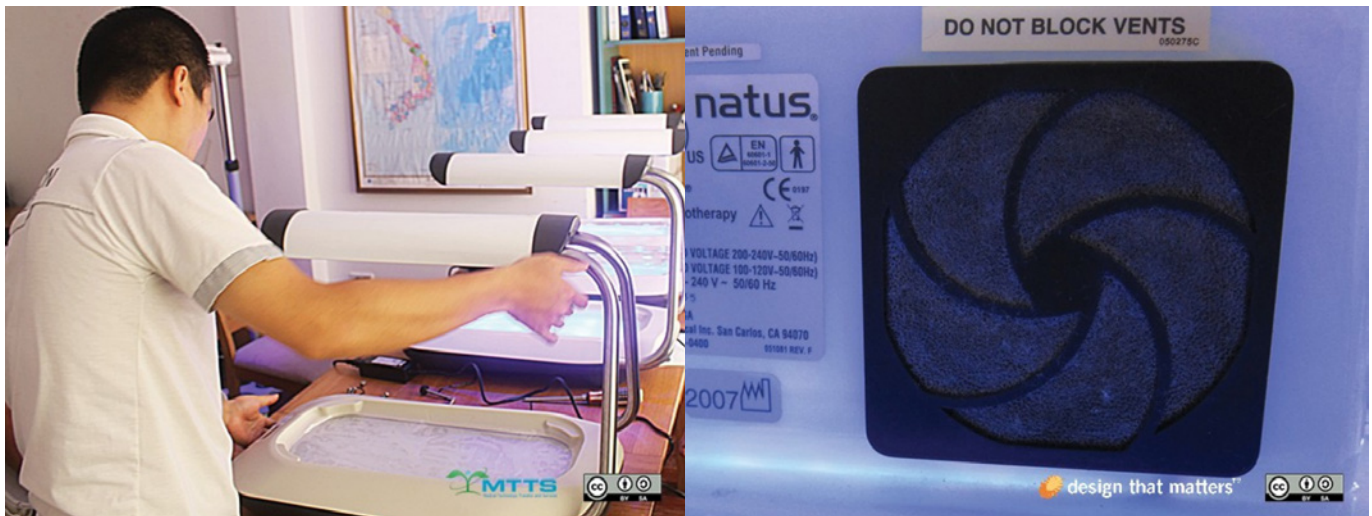
Left: Firefly manufacturer MTTS submits a series of new Firefly devices to the “burn-in test” at their offices in Vietnam. Photo courtesy Michael O'Brien of MTTS. Right: The vent for the Natus NeoBlue LED Overhead Phototherapy, one of the most popular phototherapy devices used in the United States. An internal fan helps move air through this vent to cool the electronics.
