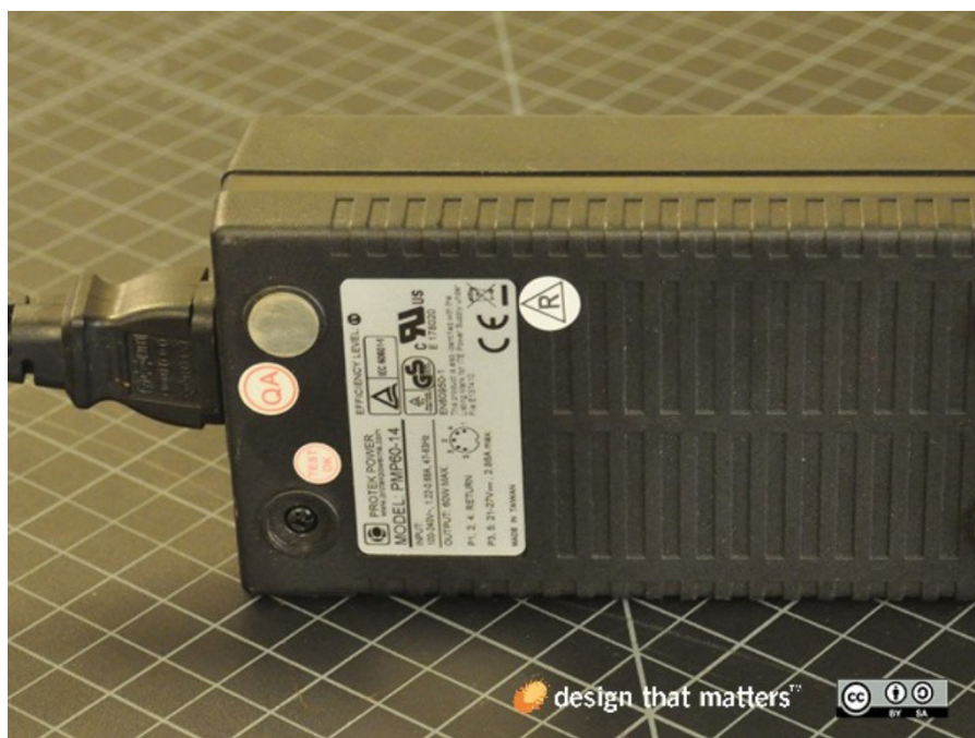
The laptop-like power supply from our Firefly clinical evaluation model prevents Firefly from burning out during a power surge, and relocates the hot power supply outside of the device and away from the baby.
