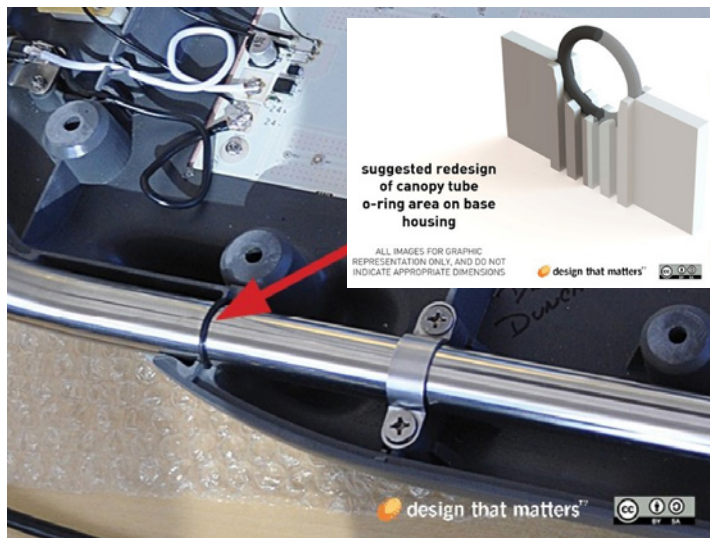
DtM used rubber o-rings to create a seal around the metal tubes where they enter the base of the device. This helps keep bugs and dust out of the device.
