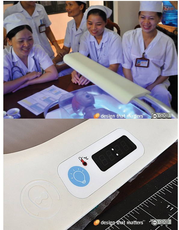
Top: Health care providers in Vietnam consider an array of different button option on paper. Bottom: The resulting simple, one-button Firefly control panel.
