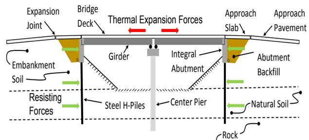
Figure 1: Schematic of Integral Abutment Bridge Cross-Section
