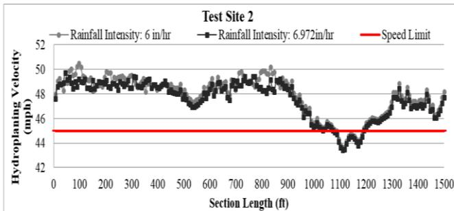
Figure 4 Hydroplaning speeds for safety evaluation (Site 2)
