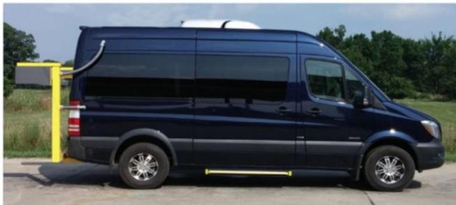
Figure 1 PaveVision 3D technology (OSU)
