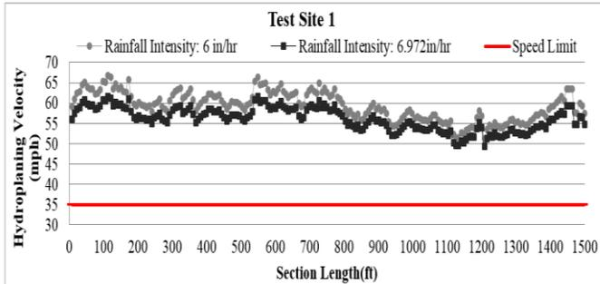
Figure 3 Hydroplaning speeds for safety evaluation (Site 1)
