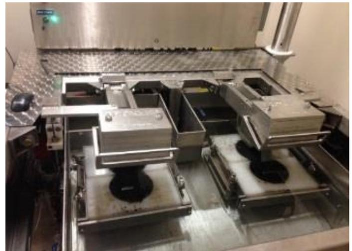
Figure 2: UNM Hamburg Wheel Tracking Device
