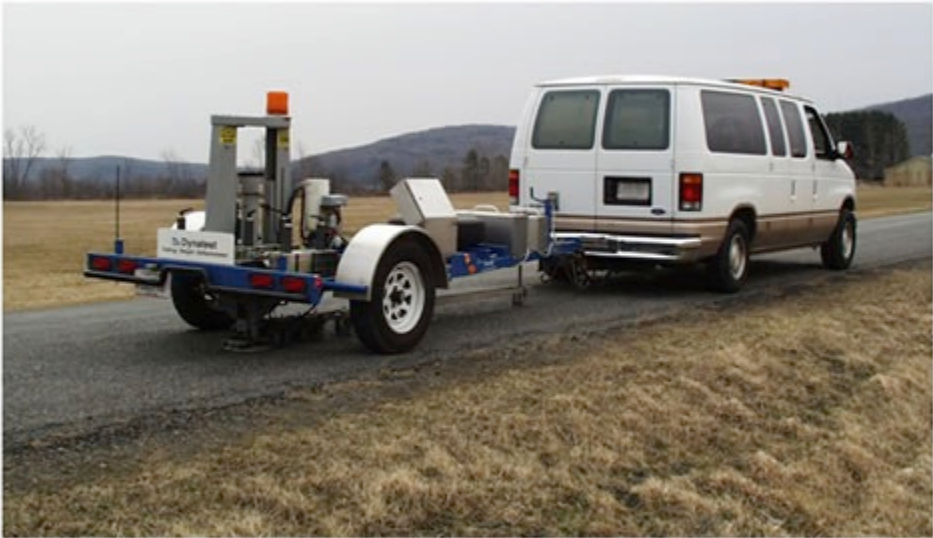
Figure 2-2. Falling Weight Deflectometer (Used with permission from FHWA).
