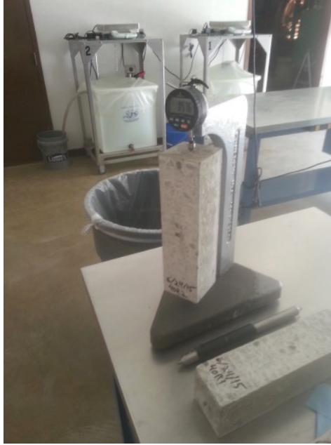
Figure 3-14. ASR prism being tested for expansion.
