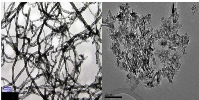
Figure 1: TEM images of MWCNTs (left) and ANPs (right).
