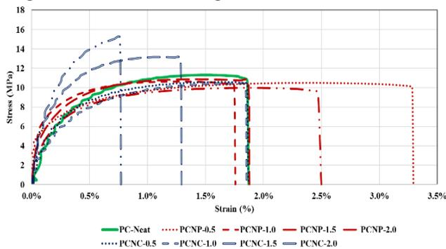
**Figure 4: Tensile stress-strain curves for MWCNTs modified PC.**
