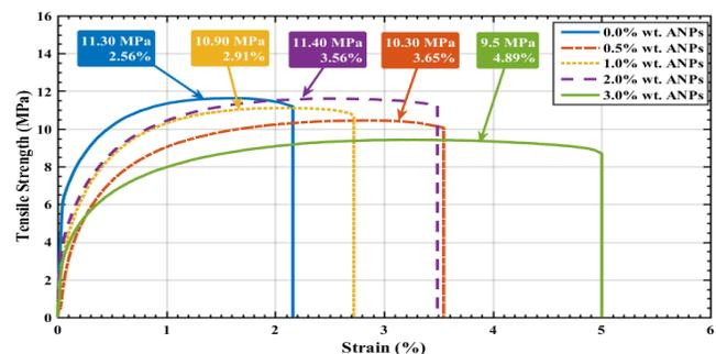
Figure 2: Tensile stress-strain curves for ANP modified PC.
