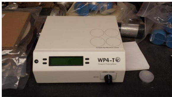
Figure 7 (a) Pressure Plate Test and (b) WP4-T Test to Construct the SWCC Curve
