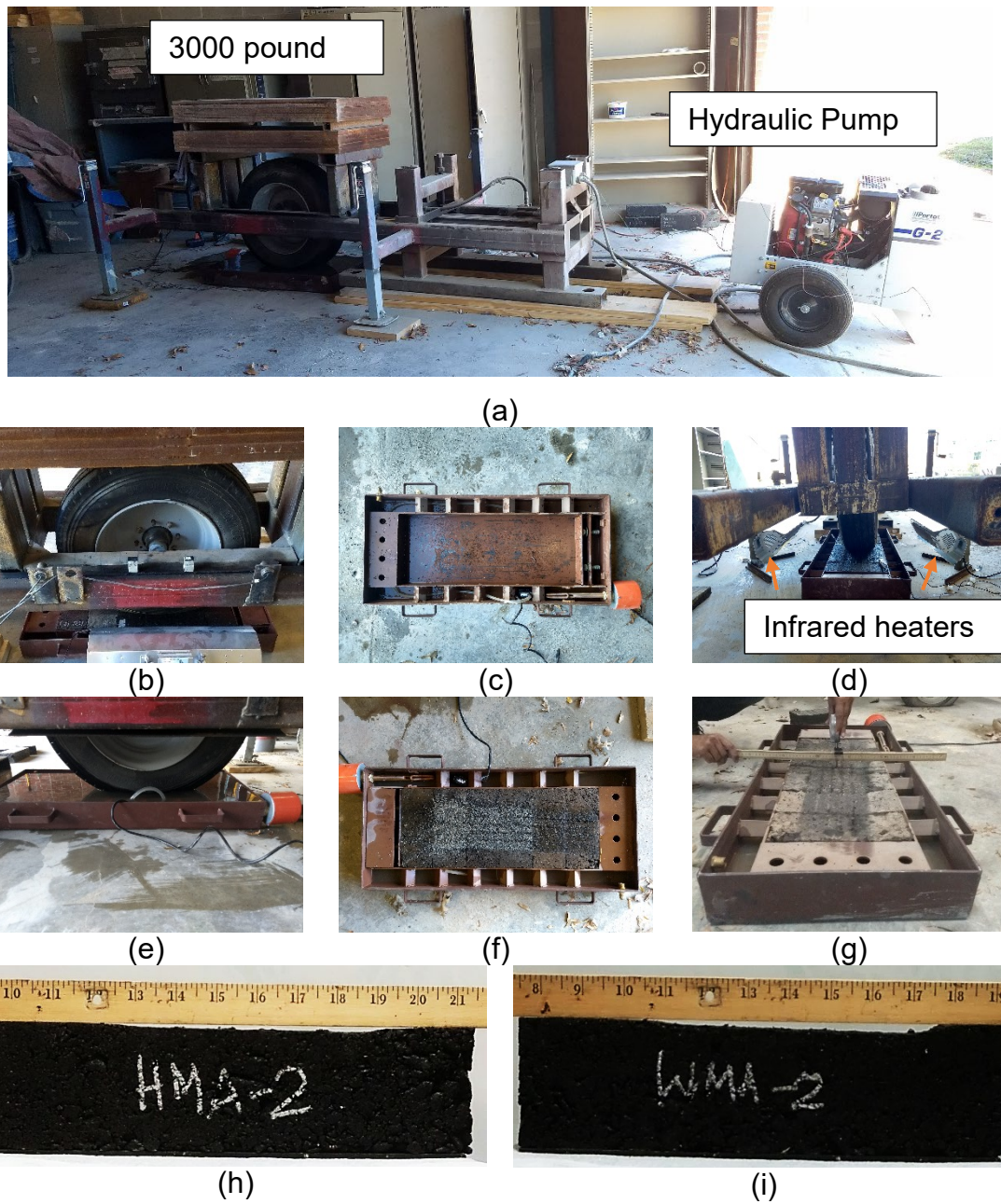
Figure 4. (a) Full view of full scale wheel load tester, (b) Sensors and magnets to control the span of wheel, (c) Specimen mold for testing, (d) Testing in dry condition is going on, (e) Submerged testing is going on, (f) Specimens in the mold after the testing is over, (g) After the testing rut depth is measured manually for individual specimen, (h) HMA specimen after rutting, (i) WMA specimen after rutting
