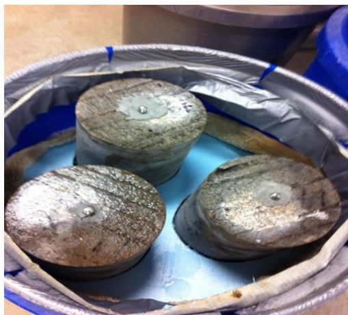
Figure 3.2. Bucket with Cores over Water
