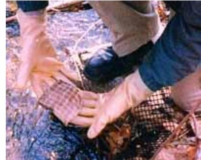
*Retrieving and rinsing the exposed Optical Brightener pad in a stream*
