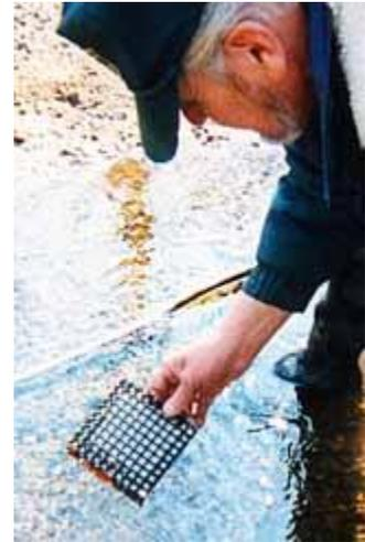
*Placing an Optical Brightener sampling device into a stream*
