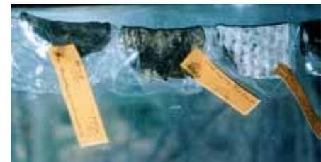
*Exposed Optical Brightener sampling pads drying on a monofilament line*
