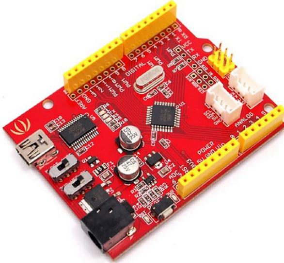
**Figure 3.** Seedeuino v 3.0 Atmega.
