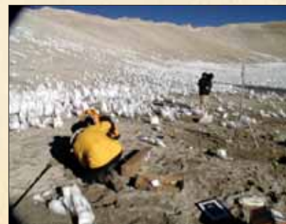
Anchoring the meteorological equipment in the permafrost at the summit of Poquentica
