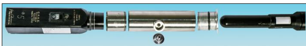
Figure 7. GRAS 42 AC Pistonphone, sleeve coupler and hydrophone
