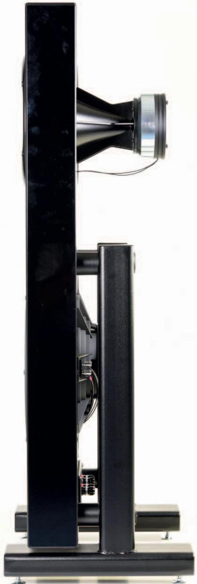
This mid-range tweeter, which was developed by Spatial in collaboration with Radian Audio, is driven by an inverted tweeter with a diameter of 10 centimeters. It plays internally on a pressure chamber which is connected to the horn through slots.
