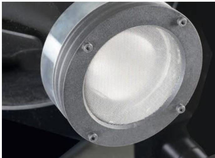
**In contrast to common compression drivers, the four inch inverted tweeter is open towards the rear. This doesn't actually amount to a true dipole characteristic, but it does bring about more airiness and high frequency energy.**
