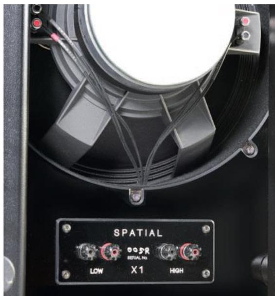
**The brachial 18 inch woofer is equipped with two voice coils that are connected in parallel. The lower as well as the mid- and high-frequency path are always actively separated and fired up over different amps.**
