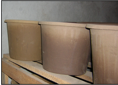
Figure 5-9: Uneven Drying (Source unknown)
