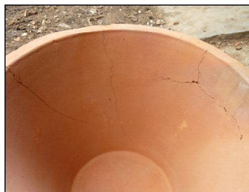
Figure 6-15: Firing/Cooling Crack (Pelita 2009)
