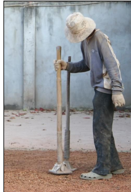
Figure 4-1: Elephant's Foot Tamper (Hagan et al. 2009)
