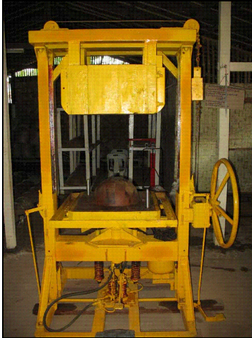
Figure 5-6: Filter Press with wooden mold, Myanmar (Thirst-Aid 2009)
