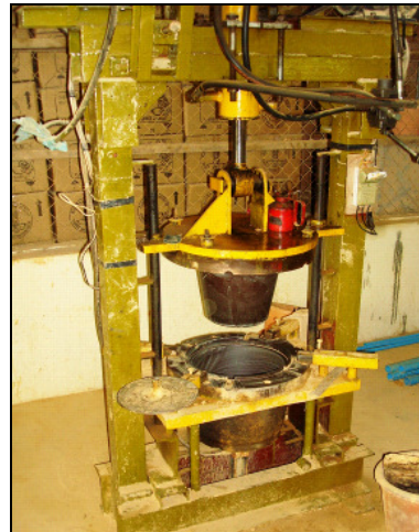
Figure 5-5: Filter Press with cast-iron mold, Cam-1 (IDECambodia 2009)
