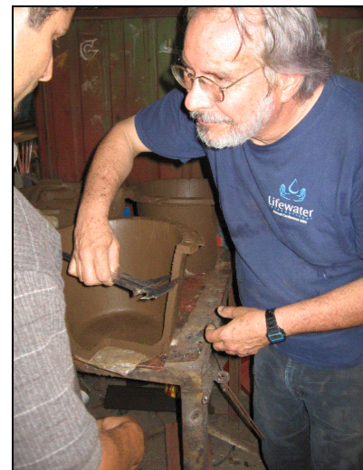
Figure 5-8: Checking Mold Alignment
