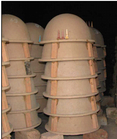
Figure 6-10: Filters Stacked for Firing, Myanmar (Thirst-Aid 2009)
