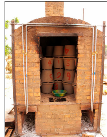
Figure 6-12: Flat bottomed filters stacked in kiln (PotterswithoutBorders 2010)
