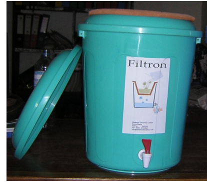
Figure 9-1: Filter Unit with Fitting Ring Ceramica Tamakloe, Ghana (Source unknown)
