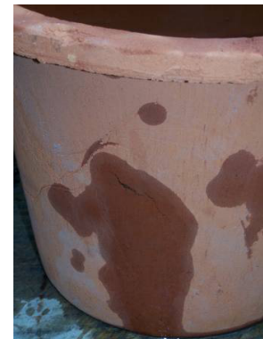
Figure 8-2: Pressure Test and Evidence of Leaks (Pillers and Diaz 2009)
