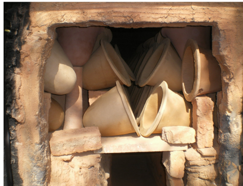
Figure 6-11: Oblong Filters Stacked for Firing (Hernandez 2010)
