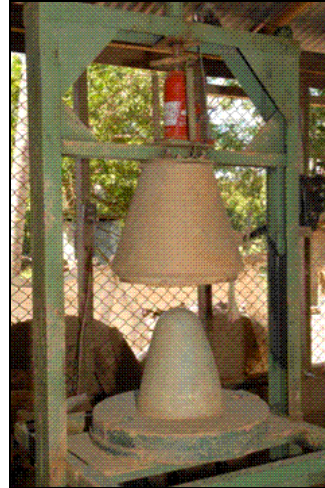
Figure 5-7: Filter Press with cement mold, DR (FilterPure 2009)
