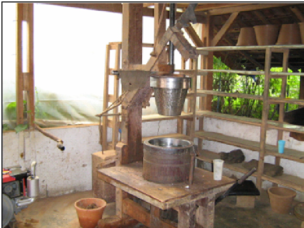
Figure 5-4: Filter Press with aluminum mold, Indo-2 (Pelita 2009)
