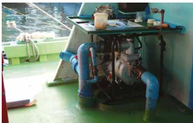
Picture 50. Electric, diesel, or gasoline-powered motors drive powerful water pumps to deliver fresh seawater to baitwells (Photo: Maldives Marine Research Centre)
