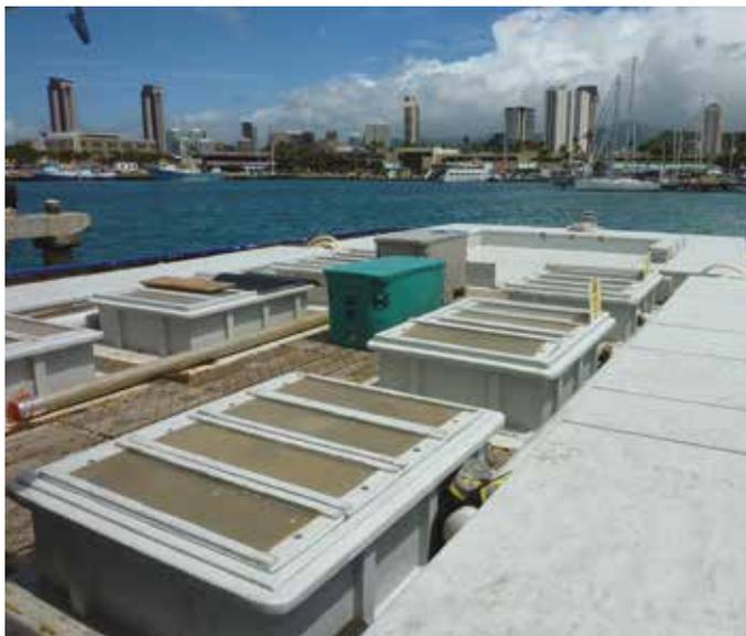
Picture 51. Six livebait wells on a pole-and-line vessel. Seawater circulation pumps maintain water levels up into the combings that discourage water sloshing out of the tanks (Photo: D. Itano)
