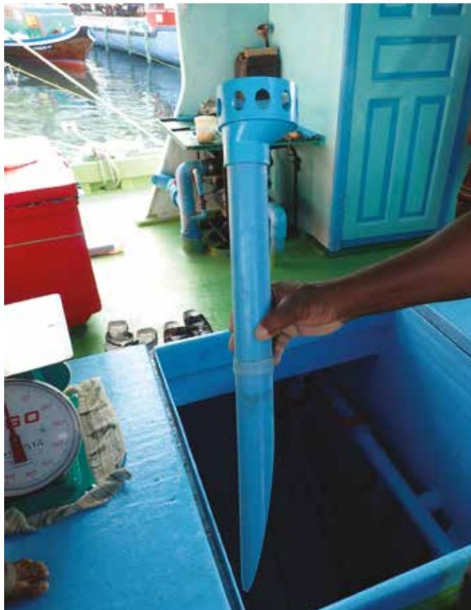
Picture 49. Manual circulation tubes are also constructed from PVC piping but also function only when the vessel is underway (Photo: D. Itano)
