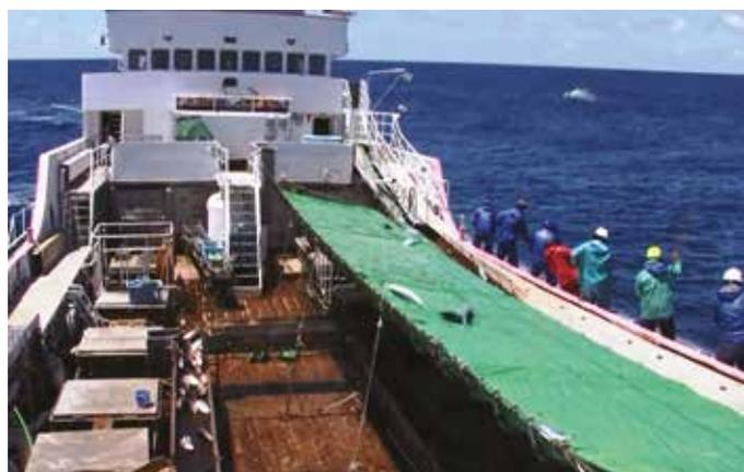
Picture 23. Skipjack flow by gravity to conveyor belt that transports fish directly to refrigerated brine well (Photo: T. Kawamoto)
