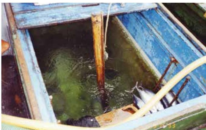
Picture 48. A bamboo pole split in half and thrust through a hole in the bottom of a baitwell helps to upwell and circulate seawater when the vessel is underway (Photo: D. Itano)
