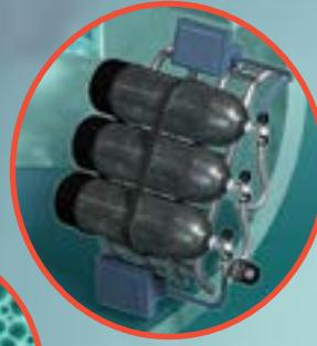
A **life-support system** includes a scrubber that removes carbon dioxide from the air and tanks of extra oxygen.
