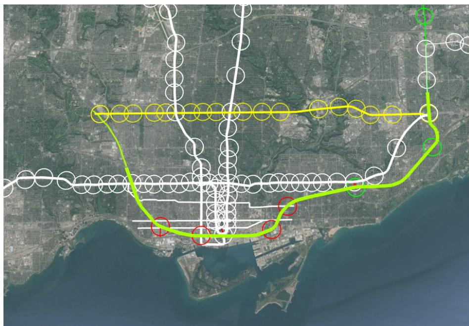
**Figure 2: Green is the corridor utilized for Quick Relief, yellow is the crosstown LRT under construction, Red circles are potential station enhancements (source: Google Maps)**
