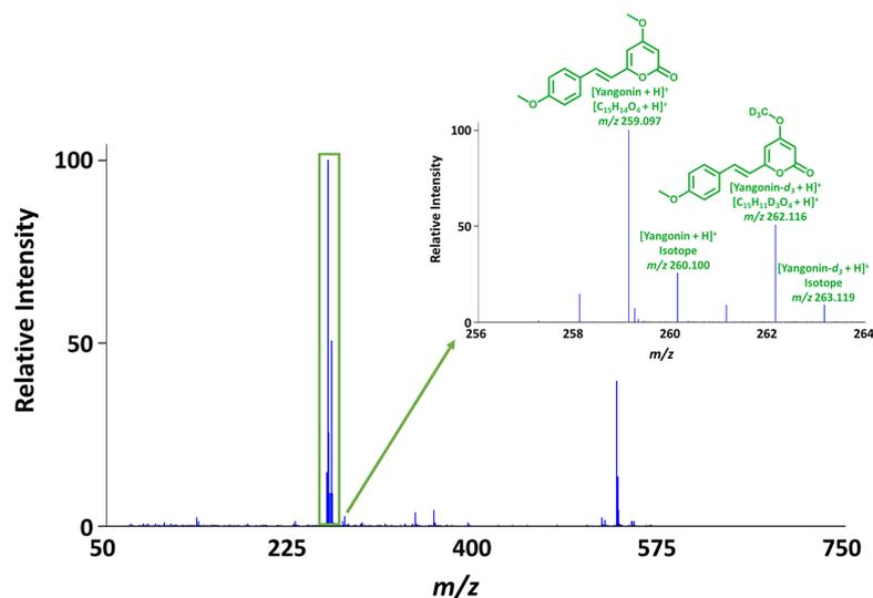
**FIGURE 4** DART-HRMS spectrum demonstrating the ratios between the yangonin and yangonin- $d_3$  peaks and the yangonin and yangonin- $d_3$  isotope peaks, all of which are in protonated form [Color figure can be viewed at [wileyonlinelibrary.com](http://wileyonlinelibrary.com)]
