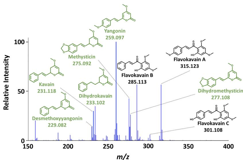
**FIGURE 1** DART-HRMS spectrum of a representative Kava product demonstrating the presence of peaks consistent with the protonated molecular weights of the six major kavalactones and three flavokavains [Color figure can be viewed at [wileyonlinelibrary.com](http://wileyonlinelibrary.com)]
