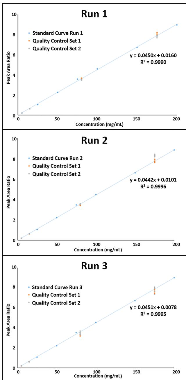
**FIGURE 5** Standard curves for yangonin quantification obtained from DART-HRMS data. All curves were developed with yangonin calibrators and yangonin- $d_3$  as an internal standard, with quality control samples to demonstrate precision and accuracy within and between runs [Color figure can be viewed at [wileyonlinelibrary.com](http://wileyonlinelibrary.com)]
