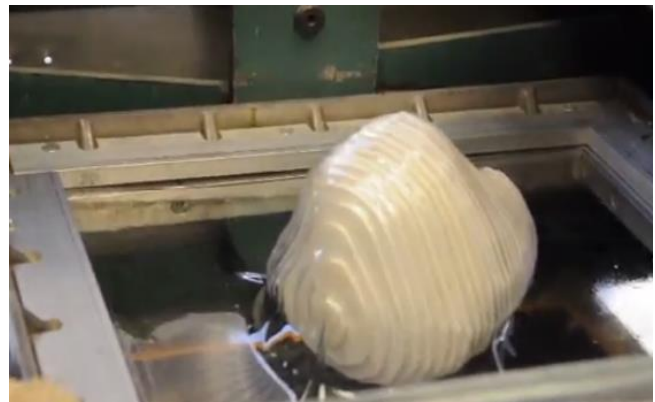
Figure 04 The mold during the prototyping process in the Vacuu-form machine
