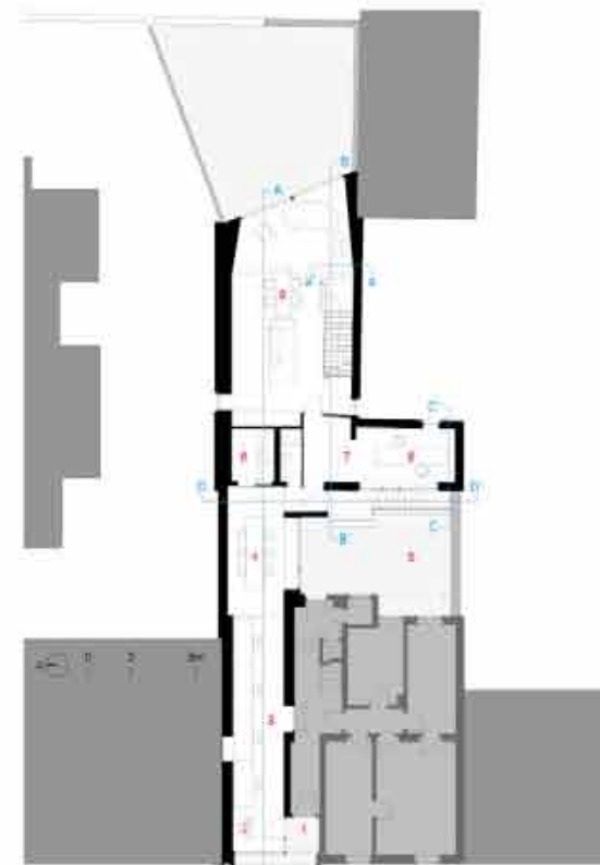
1. office entrance 2. waiting area 3. office 4. conference room 5. courtyard 6. pantry 7. wardrobe 8. office 9. kitchen+diner ground floor
