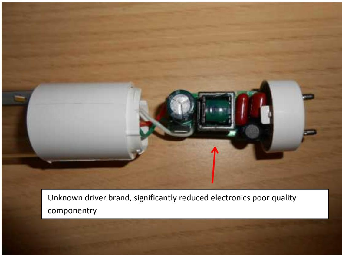
Unknown driver brand, significantly reduced electronics poor quality componentry
