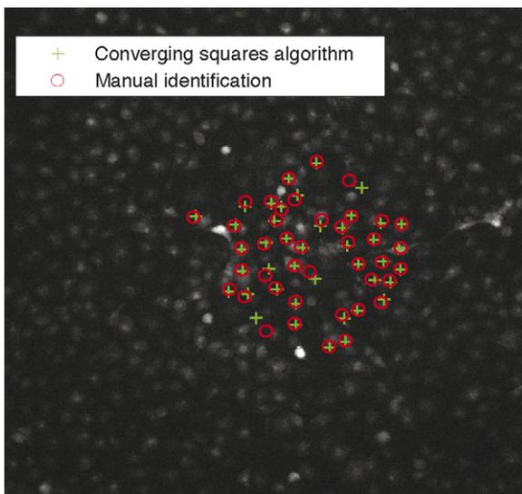
Fig. 2. Comparison of manual (crosses) and automated (circles) peak detection by the converging squares algorithm. For the algorithm, we used a square size of 10 pixels and a threshold of 80 pixels/frame (see text for details).
