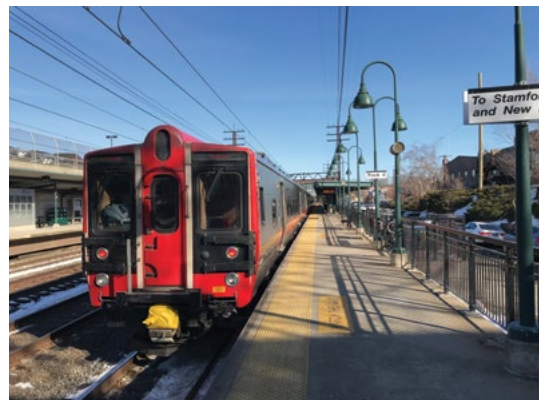
Metro North enables barrier-free universal access for riders with high-level platforms at all stations. This allows the use of modern EMUs with wide doors to speed boarding and reduce dwell time.
