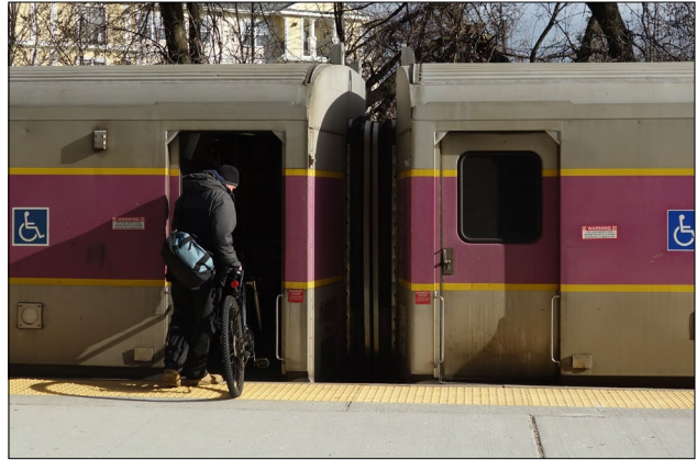
High-level platforms at stations like Salem (pictured) allow passengers to board and exit trains faster, speeding up overall trip times.
